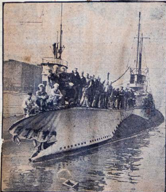
(NEWS photo) The submarine S-12 in Brooklyn navy yard after collision with car float in East river in 1926. Huge rent in bow gives it appearance of a big fish.
