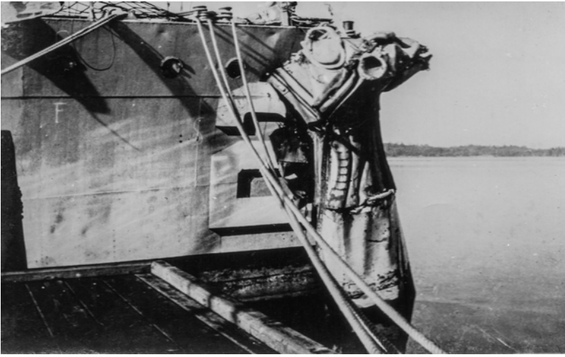
USS Whipple's damaged bow
