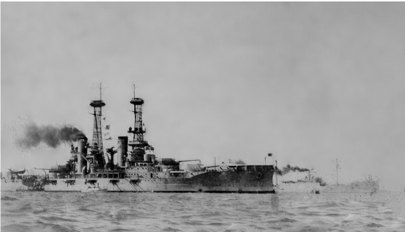
USS North Dakota (BB-29) was a dreadnought battleship commissioned in 1910, displacing 20,380 tons and with a main battery of ten 12 inch guns. She was decommissioned in 1923 as part of the Washington Naval treaty and converted to a radio-controlled target ship.
